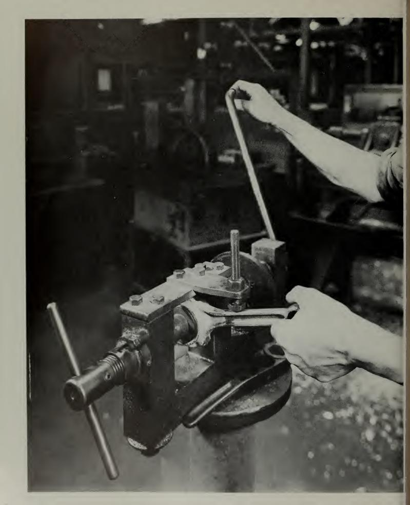
All Model A Ford and six-cylinder Chevrolet rebabbitted connecting rods require an oil groove on the face of the bearing which is cut in the shape of a figure 8 by hand operated oil groover as shown in the above picture.
